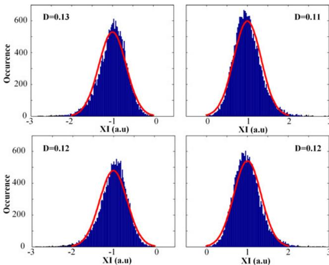
Fig. 4. Histogram of in-phase and quadrature components of the received QPSK symbols in x-polarization. Propagation over 800 km in nonlinear limited regime with the launch power of 6 dBm.
