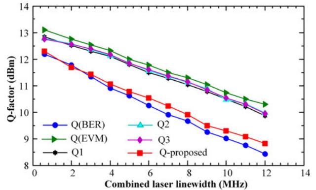
Fig. 12. Q-factor values (average over x- and y-polarization) as a function of the combined laser linewidth in 112 Gb/s PDM RGI-CO-OFDM after 4000 km of transmission; the launch power was 1 dBm.
