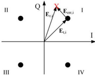
Fig. 1. Constellation diagram and error vector for a QPSK signal. Ideal constellation diagram with a received value X. Vector  $E_{t,i}$  is the transmitted signal, vector  $E_{r,i}$  is the received signal and  $E_{err,i} = E_{r,i} - E_{t,i}$  is the error vector.
