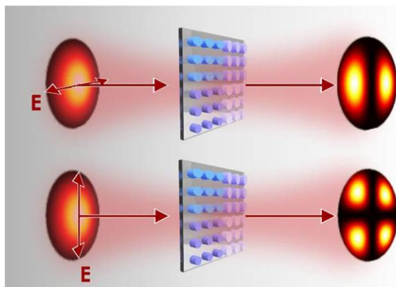
**Figure 1.** Concept of the mode multiplexing in spatial domain with metasurfaces. An all-dielectric metasurface of submicron thickness and near-unity transmission efficiency converts incoming Gaussian LP01 modes into LP11 and LP21 modes, enabling mode multiplexing.
