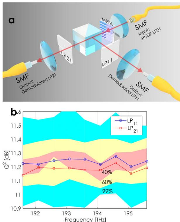
**Figure 3.** a) Experimental apparatus for the assessment of the metasurface mode multiplexer performance. b) Q factor as a function of channel frequency over the C-band with a mechanical alignment for 193.6 THz. The colored lines show the Q factor averaged over 20 repetitions for the two modes correspondingly. The colored surfaces identify the area containing the Q factor values with a probability of 40, 60, and 99%.
