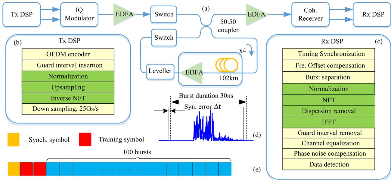
Fig. 3. (a) Schematic of the experimental setup of 10 Gbd NIS-based transmission in fibre link with EDFA-only amplification. (b)—Block diagram of the Tx DSP; (c)—block diagram of the Rx DSP; (d)—illustration of a transmitted burst with a duration of 30 ns carrying 120 bits (60 QPSK symbols) and illustration of synchronization error. (e)—structure of the transmitted signal, including one synchronization symbol, two training symbols for channel estimation and 100 OFDM NIS-based bursts.
