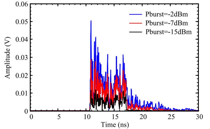
Fig. 4. Comparison of output signals of the INFT block given the same input 10 Gbd OFDM waveform with different power levels.
