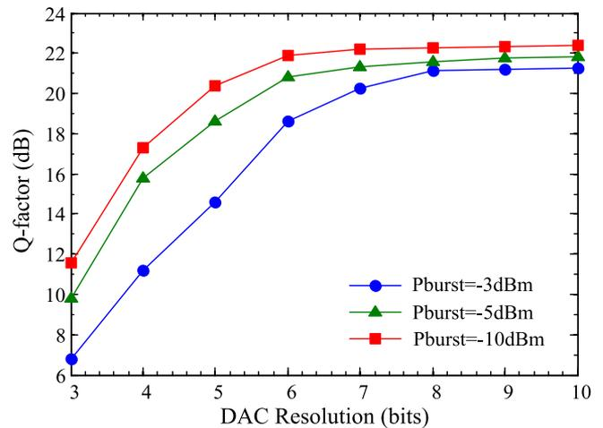
Fig. 7. Simulated back-to-back performance of NIS-based 10 Gbd OFDM system sampling at 25 Gs/s with different values of the burst power the Tx DAC resolutions.
