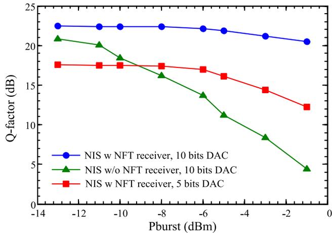
Fig. 5. Simulated back-to-back performance of NIS-based 10 Gbd OFDM system at 25 Gs/s with and without NFT receiver. The DAC resolutions are 5 and 10 bits, no noise was added.
