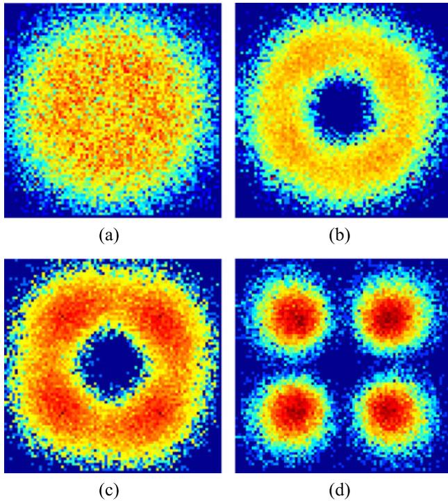
Fig. 9. Constellation diagrams at the burst power of  $-5$  dBm after 4080 km of transmission distance, (a)—before dispersion removal, (b)—before channel estimation, (c)—before phase noise compensation, (d)—final constellation after phase noise compensation.
