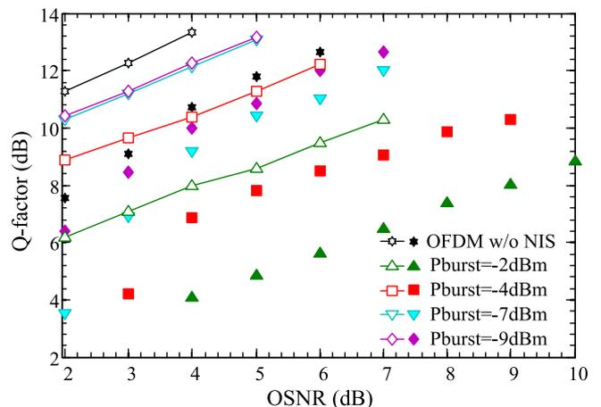
Fig. 8. Back-to-back performances of 10 Gbd OFDM and NIS-based OFDM systems for different burst power values. Closed symbols are experimental data. The solid lines with open symbols are simulation results, the DAC resolution was set to 5 bits.
