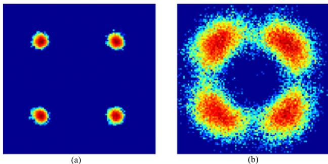
Fig. 6. Received constellations of NIS-based 10 Gbd OFDM system at 25 Gs/s with and without NFT receiver,  $P_{\text{burst}} = -3$  dBm.
