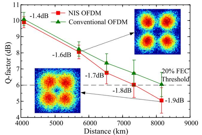
Fig. 11. Optimum Q-factor as functions of the transmission distance. The numbers are power correction values for each distance at the optimum burst power.
