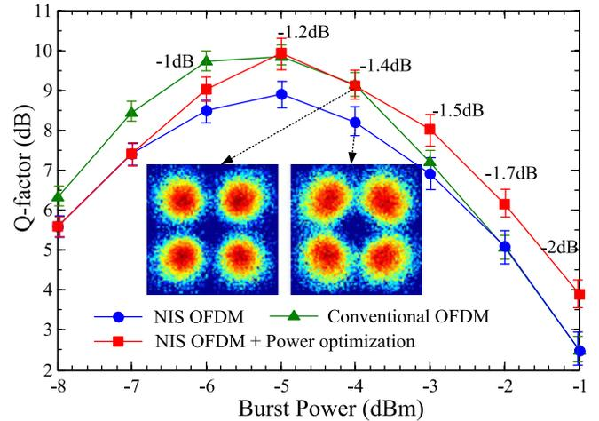
Fig. 10. Q-factor as a function of the burst power after 4080 km. The numbers are power correction values for each burst power value.
