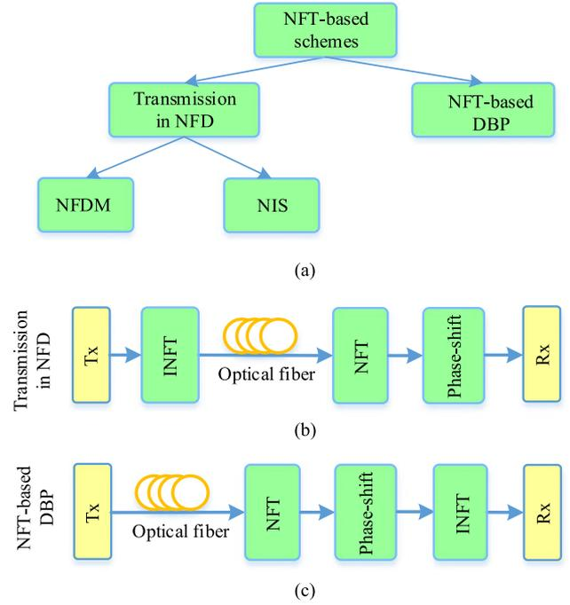
Fig. 2. (a) Basic designs of NFT-based transmission systems; (b) transmission in the NFD; (c) NFD based DBP (NFD-DBP).
