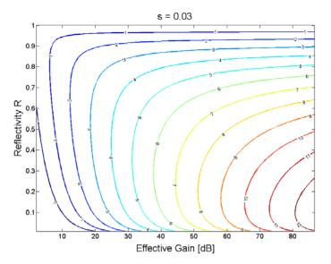
Fig. 2. Contour plot of the normalized energy  $E / E_{sat}$  in the plane (gain, R); here s = 0.03.
