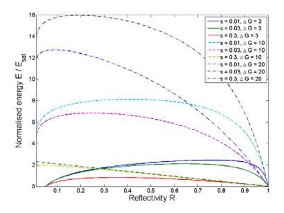
Fig. 4. Normalized energy  $E/E_{sat}$  vs. the reflectivity R for different gains and s.
