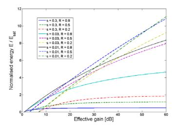
Fig. 3. Normalized energy  $E/E_{sat}$  as a function of an effective gain for different R and s.
