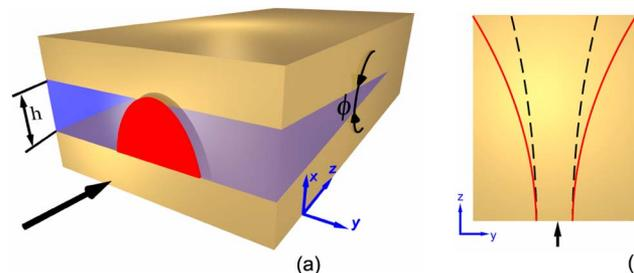
Fig. 1. (Color online) (a) Schematic of a tapered metal–dielectric–metal slot waveguide. (b) Schematic of the plasmonic beam propagation in linear (dashed curve) and nonlinear (solid curve) regimes.
