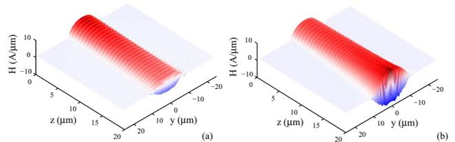
Fig. 3. (Color online) Magnetic field profiles at the metal-dielectric interface for (a) nonlinear untapered ( $\phi = 0^\circ$ ) and (b) nonlinear tapered ( $\phi = 1.6^\circ$ ) waveguides. Field profiles are plotted up-till few microns from the taper tip.
