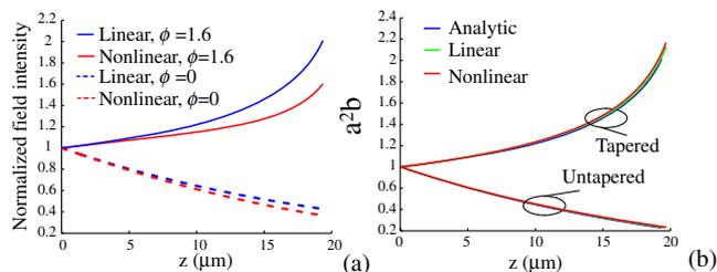
Fig. 4. (Color online) (a) Evolution of the beam amplitude with propagation obtained from the analytical theory for all studied cases. The fields are normalized to the initial amplitude  $a(0)$ . (b) Evolution of product  $a^2b$  with propagation for tapered and untapered waveguides, for different input amplitudes.
