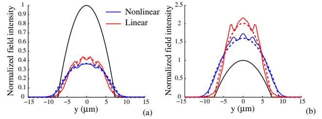
Fig. 2. (Color online) Beam cross-sections for (a) untapered and (b) tapered waveguides, respectively, after 20  $\mu\text{m}$  of propagation. Solid curves correspond to numerical results, whereas dashed are our analytic predictions. Solid parabolic curve corresponds to the input beam profile.
