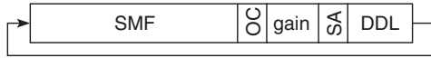
FIG. 3. Schematic model for the laser. SMF, single-mode fiber; OC, output coupler; SA, saturable absorber; DDL, dispersive delay line.
