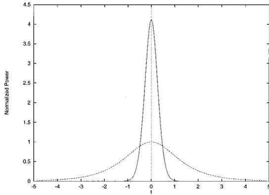
FIG. 1. Shape of the soliton with Gaussian tails. It is plotted power distribution  $|F(t)|^2$  (normalized to the peak power of the fundamental soliton) in the solutions of Eq. (1) with  $k=0.5$  for different values of  $a$  vs normalized time  $t$ . Dashed line, soliton of the NLSE ( $a=0$ ); solid line, the soliton with Gaussian wings for  $a=10$ .
