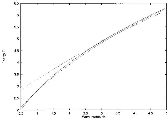
FIG. 3. The energy of the soliton as a function of the wave number  $k$  for different  $a$ : solid line for  $a=0$  (fundamental soliton) dashed line close to solid one is for  $a=1$ , and dotted curve for  $a=10$ . Monotonic growth of the energy with increasing of  $k$  determines the stability of the soliton with Gaussian wings.
